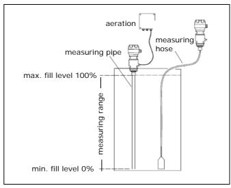
Various methods can be used to install the hydrostatic level transmitter to containers and tanks:
